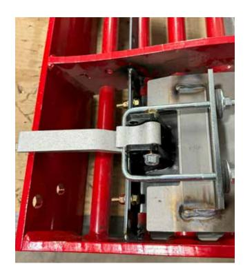
4. Hook u-bolt into latch and close latch, tighten u-bolt nuts as required to create firm closure
