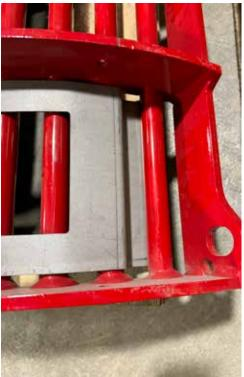
3. Hook cover plate on last rung on left concave, on right concave slide end between 1st and second rung
