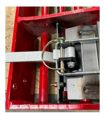
5. Insert pin to lock latch down
