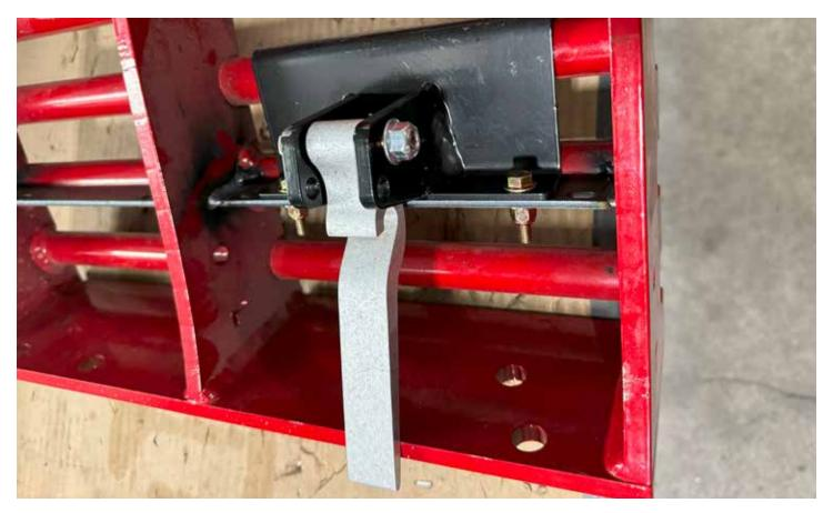
2. Install latch to bracket with supplied flange bolt
